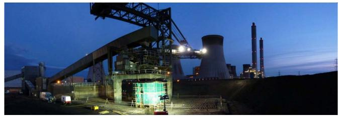
The Boom Stacker is part of the coal handling plant sited at West Burton Coal Fuelled Power Station. It is responsible for handling the majority of coal deliveries on the site, and does so using a system comprising of a slewing conveyor & boom.
